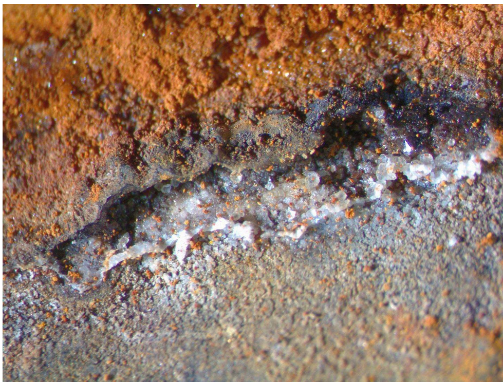
Deposit of white cubic particles located at the waterline of a cauldron's foot from Herbeumont. Optical microscopy image 10709.
