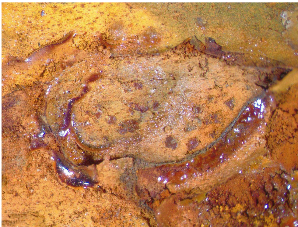
Imprint of a Ziplock bag on the surface of a saw blade from Herbeumont Castle, along with a detail of the shiny substance.
