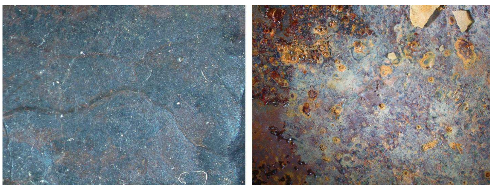
Corrosion beneath the consolidated surface of a ladle from Renaud Castle (a) and Herbeumont Castle (b).
