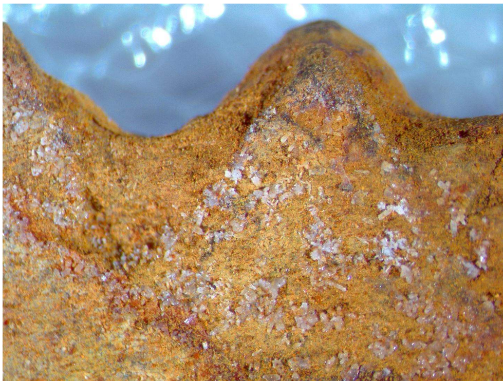
White needles and cubic particles on a saw blade from Herbeumont. Optical microscopy image 10651.
