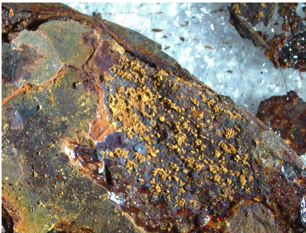
Flakes detaching from the surface of a horseshoe at Wanze Golf. Optical microscopy image 10313.
