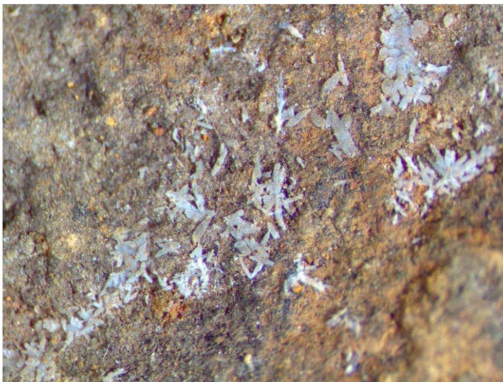
Drusy aggregates of small white needles on a cauldron fragment from Herbeumont. Optical microscopy image 10637.
