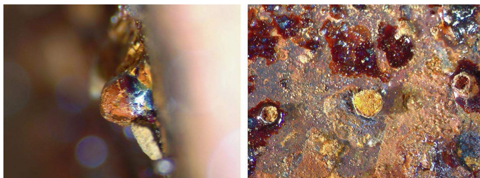
Elongated particles seem to 'grow' from the surface of a cauldron from Herbeumont. Optical microscopic images 10533 and 10534.
